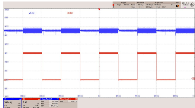
Figure 64 – Transient Response. 265 VAC, 9 V, 0% – 100% Load Step. V_{MIN} : 8.957 V, V_{MAX} : 9.434V. C1: V_{OUT} , 500 mV / div. C2: I_{OUT} , 1 A / div. Time: 200 ms / div.
