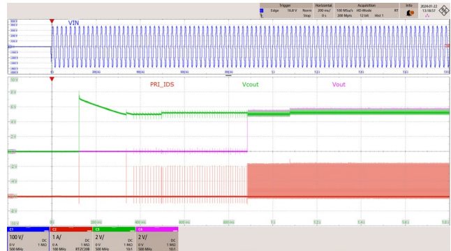
Figure 54 – Output Voltage at Start-up. 265 VAC, 5 V, 3 A Load. C1: V_{IN} , 100 V / div. C2: Primary I_{DS} , 1 A / div. C3: V_{COUT} , 2 V / div. C4: V_{OUT} , 2 V / div. Time: 200 ms / div.
