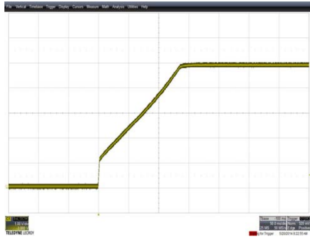
Figure 18 – Start-Up Profile, 115 VAC. Full Load. 1 V / div., 50 ms / div.
