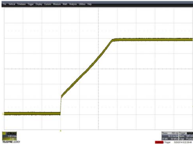
Figure 17 – Start-Up Profile, 85 VAC. Full Load. 1 V / div., 50 ms / div.
