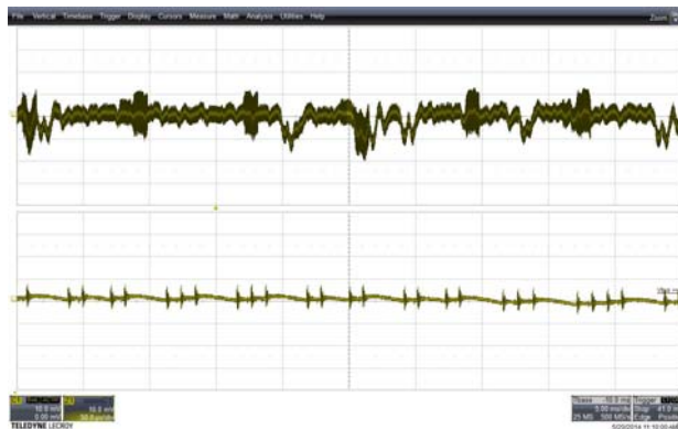
Figure 33 – Ripple, 260 VAC, Full Load. Upper :5 ms, 10 mV / div. Lower: 50 μs, 10 mV / div.
