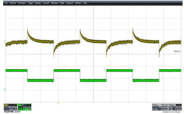
Figure 24 – Transient Response, 260 VAC, 800 mA to 1600 mA. 100 ms / div. Upper: V_{OUT} 100 mV / div. Lower: I_{OUT} 1 A / div.
