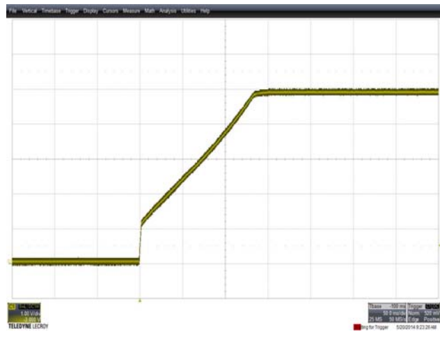
Figure 20 – Start-Up Profile, 260 VAC. Full Load. 1 V / div., 50 ms / div
