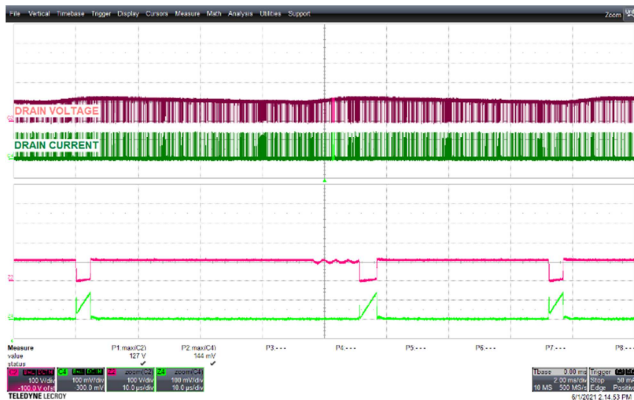
Figure 19 – 90 VAC 60 Hz. CH2: V_{DRAIN} , 100 V / div., 2 ms / div. CH4: I_{DRAIN} , 100 mA / div., 2 ms / div. V_{DRAIN(PEAK)} : 127 V; I_{DRAIN(PEAK)} : 144 mA.
