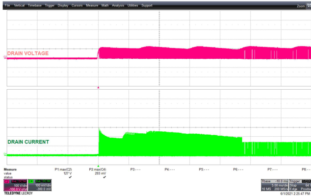
Figure 17 – 90 VAC 60 Hz. CH2: V_{DRAIN} , 100 V / div., 5 ms / div. CH4: I_{DRAIN} , 100 mA / div., 5 ms / div. V_{DRAIN(PEAK)} : 127 V; I_{DRAIN(PEAK)} : 293 mA.
