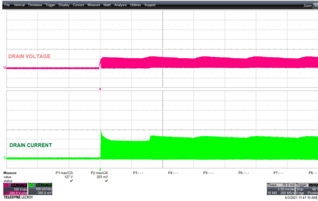
Figure 21 – 90 VAC 60 Hz. CH2: V_{DRAIN} , 100 V / div., 5 ms / div. CH4: I_{DRAIN} , 100 mA / div., 5 ms / div. V_{DRAIN(PEAK)} : 127 V; I_{DRAIN(PEAK)} : 293 mA.
