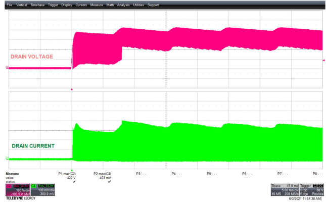
Figure 22 – 300 VAC 60 Hz. CH2: V_{DRAIN} , 100 V / div., 5 ms / div. CH4: I_{DRAIN} , 100 mA / div., 5 ms / div. V_{DRAIN(PEAK)} : 422 V; I_{DRAIN(PEAK)} : 403 mA.
