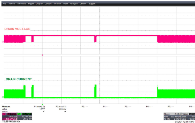
Figure 23 – 90 VAC 60 Hz. CH2: V_{DRAIN} , 100 V / div., 500 ms / div. CH4: I_{DRAIN} , 100 mA / div., 500 ms / div. V_{DRAIN(PEAK)} : 127 V; I_{DRAIN(PEAK)} : 224 mA.
