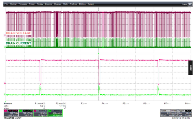
Figure 20 – 300 VAC 60 Hz. CH2: V_{DRAIN} , 100 V / div., 2 ms / div. CH4: I_{DRAIN} , 100 mA / div., 2 ms / div. V_{DRAIN(PEAK)} : 432 V; I_{DRAIN(PEAK)} : 177 mA.
