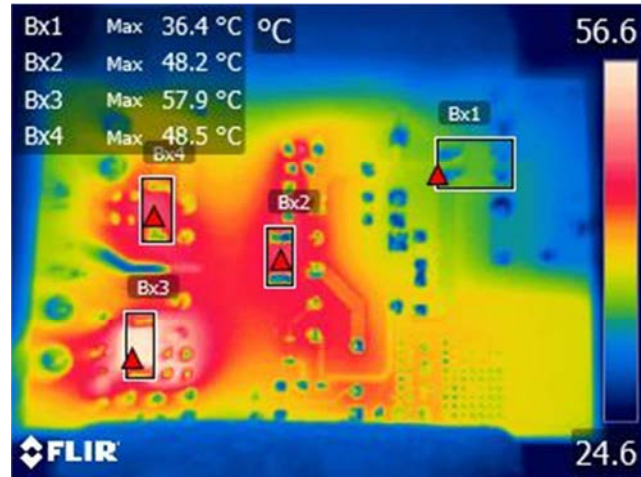
Figure 84 – Ambient = 24.6 °C. Bx1, BR1: 36.4 °C. Bx2, D1: 48.2 °C. Bx3, D3: 57.9 °C. Bx4, D4: 48.5 °C.
