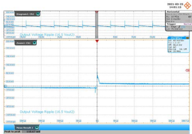
Figure 30 – 85 VAC Input. Vertical: 40 mV / div. Horizontal: 4 ms / div., 50 μs / div. 16.5 V OUT2 Ripple: 110.67 mV PK-PK .
