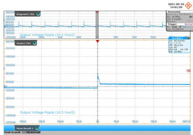
Figure 32 – 115 VAC Input. Vertical: 40 mV / div. Horizontal: 4 ms / div., 50 μs / div. 16.5 V OUT2 Ripple: 98.024 mV PK-PK .
