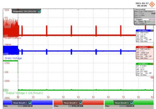
Figure 72 – 115 VAC Input. 16.5 V OUT1 : 5 V / div., 1 s / div. Drain Current: 500 mA / div. Drain Voltage: 500 V / div.
