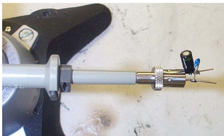
Figure 20 – Oscilloscope Probe with Probe Master ( www.probemaster.com ) 4987A BNC Adapter. (Modified with wires for ripple measurement, and two parallel decoupling capacitors added.)
