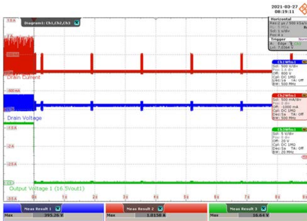
Figure 71 – 85 VAC Input. 16.5 V OUT1 : 5 V / div., 1 s / div. Drain Current: 500 mA / div. Drain Voltage: 500 V / div.
