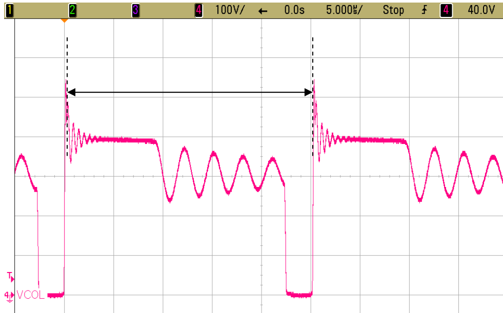
Figure 36: Q1 Collector Voltage Waveform with 100% Load
