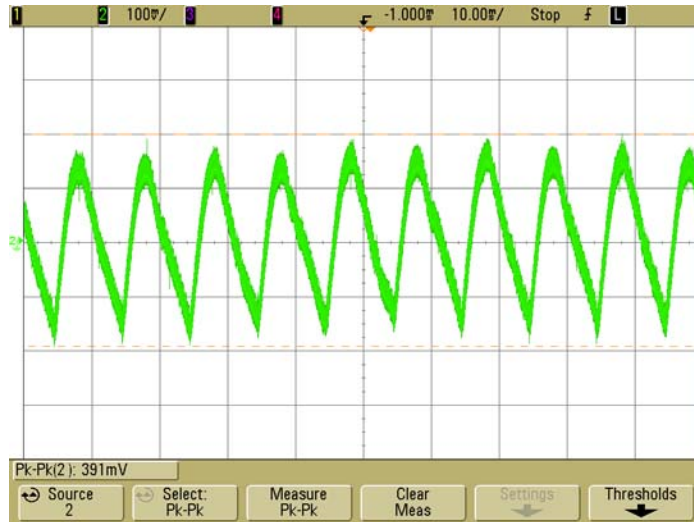
Figure 12: 100 Hz Output Voltage Ripple with 1000 \mu\text{F} Extra Load Capacitance
