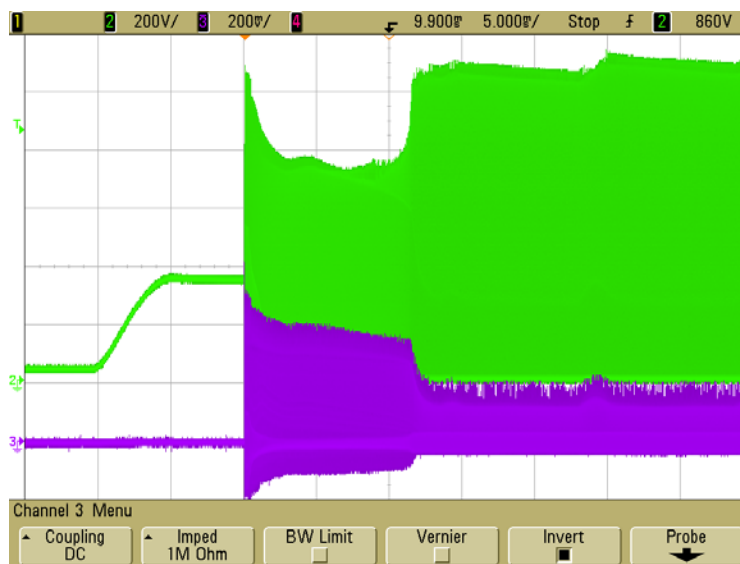
Figure 14: Start-up Switching Transistor Voltage and Current, 5 ms/div
