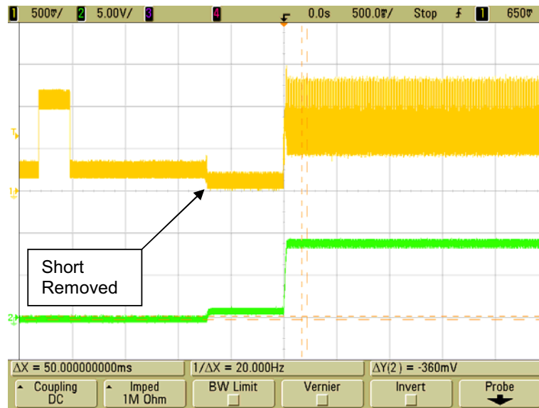
Figure 24: Output Short-Circuit Recovery With 1000 \mu F Extra Load Capacitance. Short Circuit Current (CH1 at 0.5 A/div) and Output Voltage (CH2 at 5 V/div). Timebase is 0.5 s/div.
