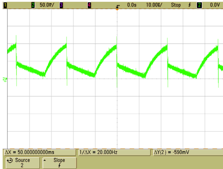
Figure 21: Switching Frequency Ripple Without Additional Load Capacitance (CH2 at 50 mV/Div). Timebase is 10 \mu s/div.
