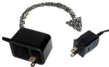
Figure 2: Size (and cost) reduction moving from a linear PSU to an RDFC SMPS solution
